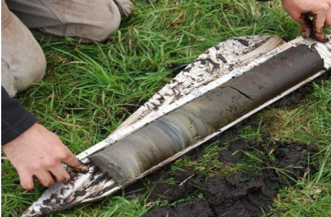
Fig 2: Collecting Soil Sample for Preliminary Soil Exploration
